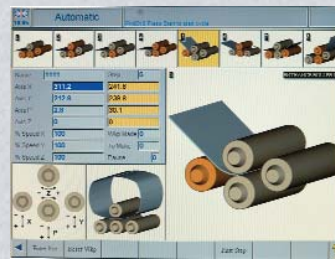
Precise conical and poly-centric bending with CNC controls
