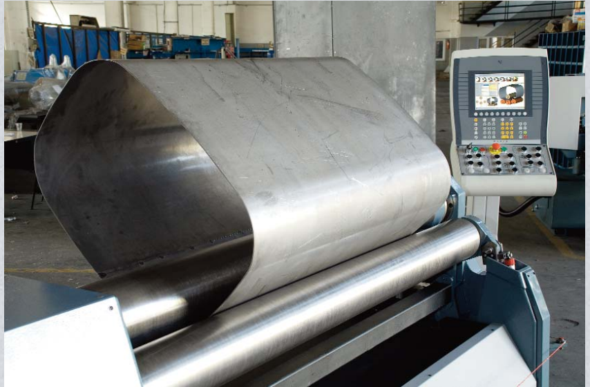
Precise conical and poly-centric bending with CNC controls
