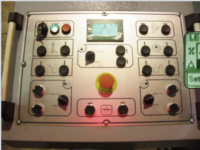
Standard 4-Roll Control with 6 Digital Readouts on Touch Screen Panel with Multiple Programmable Pass Points
