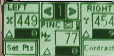
Standard 4-Roll Control with 6 Digital Readouts on Touch Screen Panel with Multiple Programmable Pass Points
